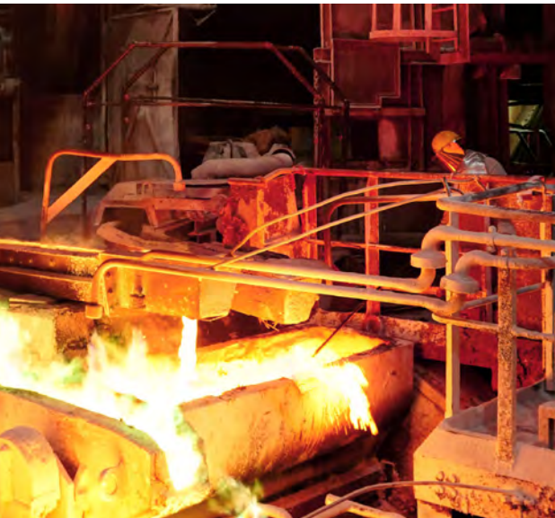
Technically feasible: using hydrogen instead of natural gas for carbon-neutral anode production.
